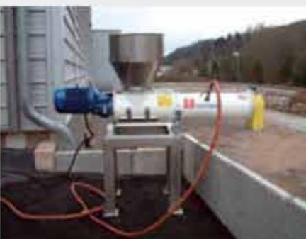
**Conditioners for Ceramic Dust***Befeuchtungsmischer für Keramikstäube**Humidificateurs de poussière céramique**Umidificatori di polvere da ceramica*
