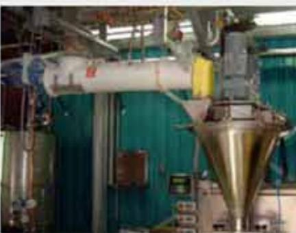
**Dust Conditioners***Staubbefeuchtungsmischer**Humidificateurs de poussière**Umidificatori di polvere*
