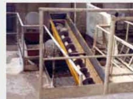
Screw Conveyors for Fresh Concrete
