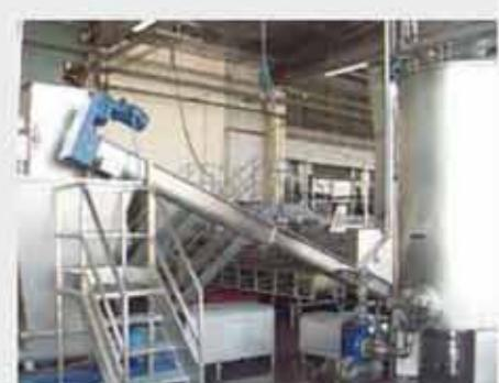
Stainless Steel Trough Screw Conveyors
