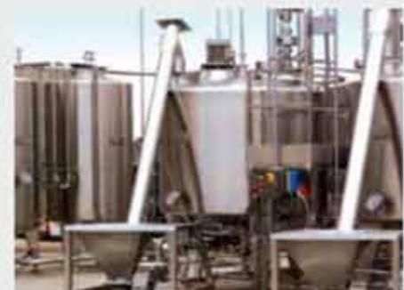
Stainless Steel Tubular Screw Conveyors
