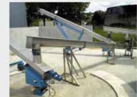
Stainless Steel Shaftless Spiral Conveyors
