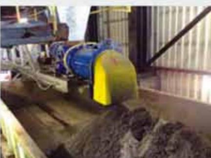
**Dust Conditioners***Staubbefeuchtungsmischer**Humidificateurs de poussière**Umidificatori di polvere*
