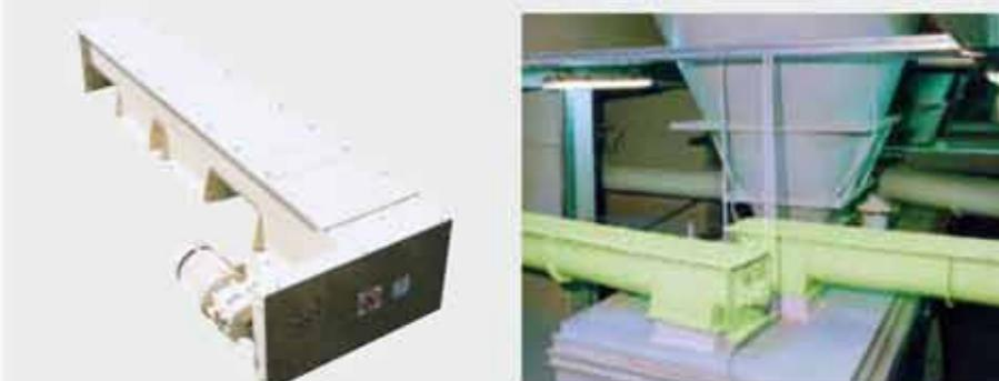
$\varnothing = 150 \sim 400 \text{ mm (} 6'' \sim 16''\text{)}$     $Q_{\max} = 105 \text{ t/h cereals / flour}$
