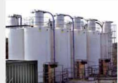
Filtration surface area: 1 ~ 48 m<sup>2</sup> (11 ~ 517 sq ft) Air volume: 60 ~ 4,500 Nm<sup>3</sup>/h (35 ~ 2,650 cfm)
